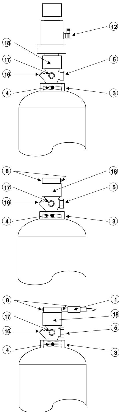
The valves B480 are activated by electrical or pneumatic actuator (tripping mechanism/release unit) on the valve. The electrical actuator must be reset after a triggering with the tensioning device (reset device). Otherwise the valve is immediately activated at the assembly of the actuator.
