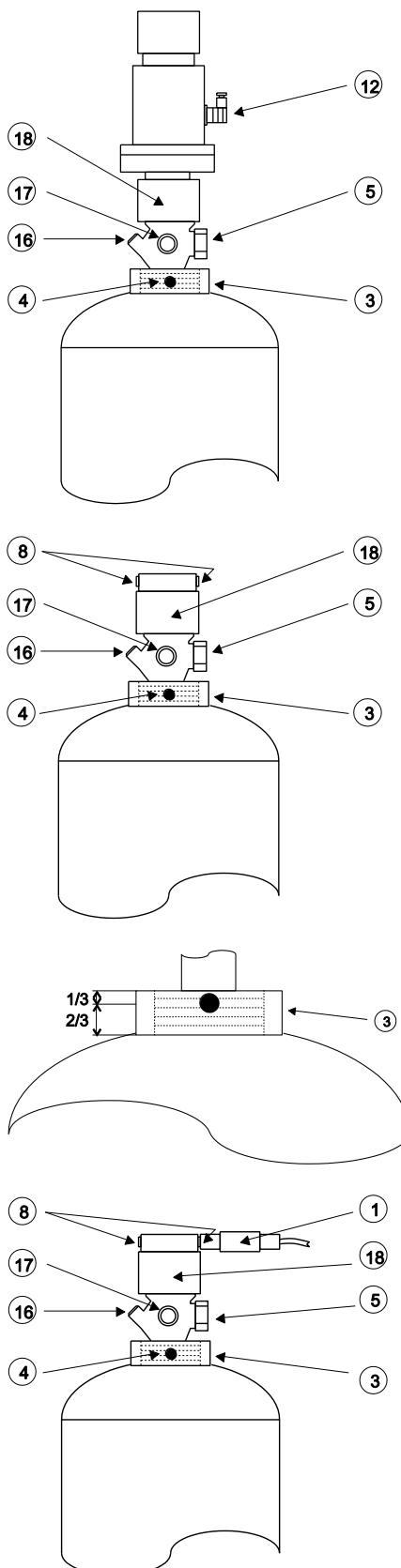
The valves B480 are activated by electrical or pneumatic actuator (tripping mechanism/release unit) on the valve. The electrical actuator must be reset after a triggering with the tensioning device (reset device). Otherwise the valve is immediately activated at the assembly of the actuator.
